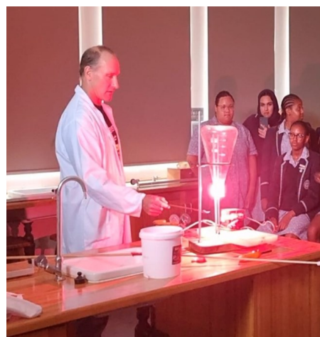
Dr Rubidge demonstrating atomic emission using an electric arc to excite strontium
